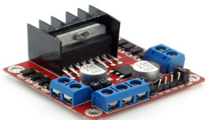
Fig 3: L298N Motor driver
