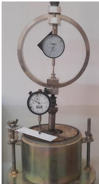
**Fig. 1.** Beginning of a CBR test (GTX is put on top of the sand).
