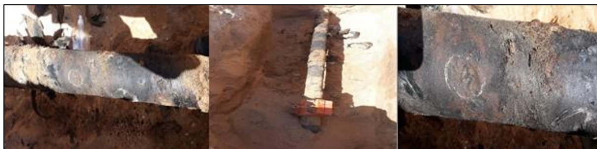
Figure 3: Perforation Level of 4" Pipe
