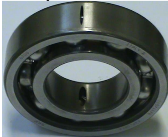
Figure 2. Ball bearing with artificial spalls.
