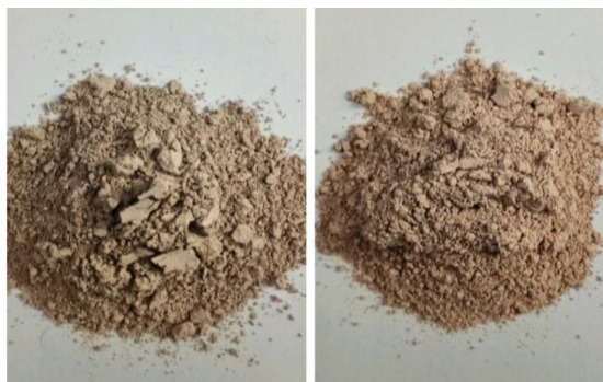
Figure 4 - kaolin on the left and metakaolin on the right.
