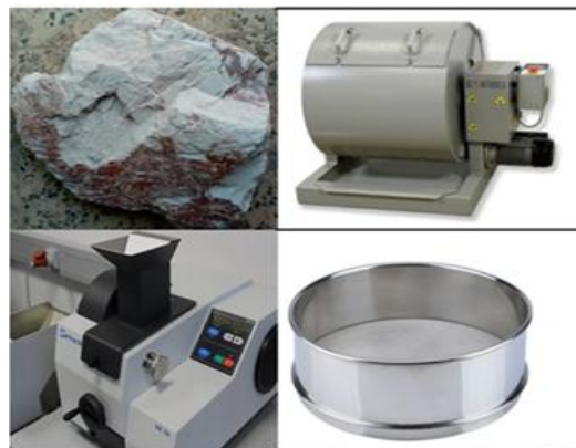
Figure 1 - Device for the preparation of metakaolin.
