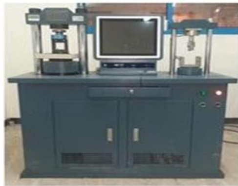
Fig.4: Flexural test set-up
