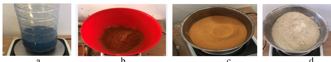
Fig. 2- Materials used in Formulation; a: Resin, b: Red clay, c: Dune sand (SD),
