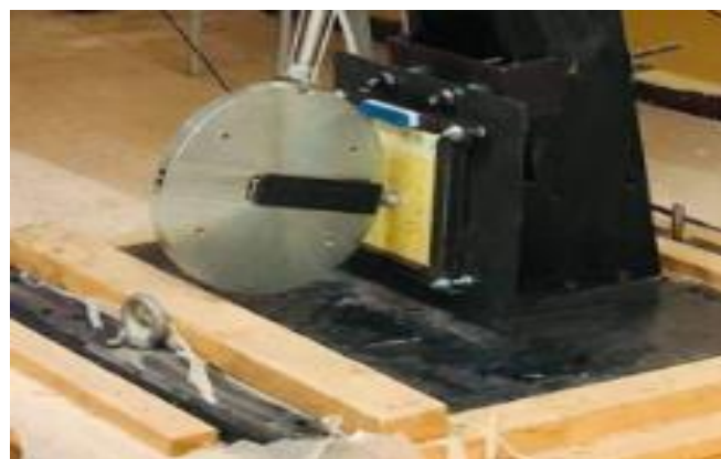
Fig.3: Collision between the collider and the embedded sample
