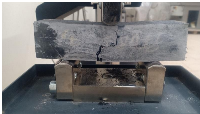
FIGURE 3. Flexural strength test three point.
