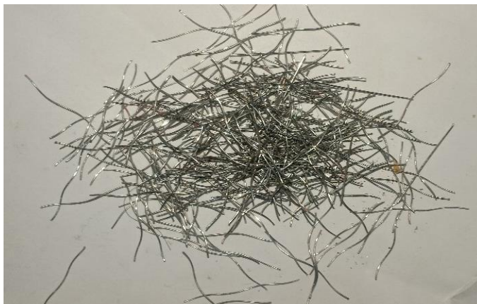
Figure 2 .waste steel fiber length 20 mm.
