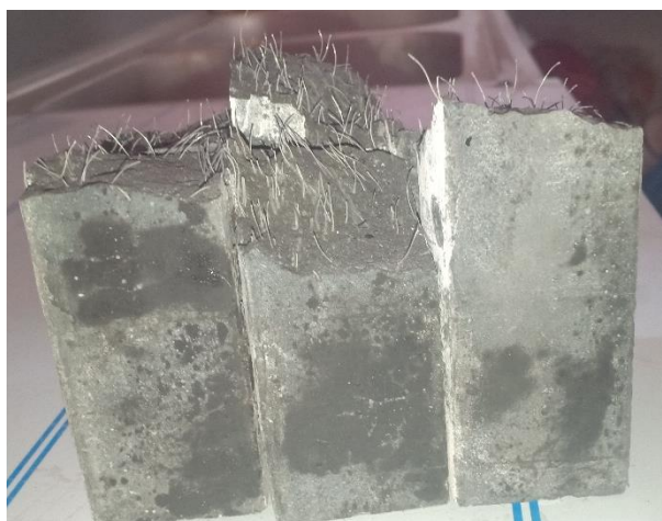
FIGURE 7.Orientation and distribution of fibers.
