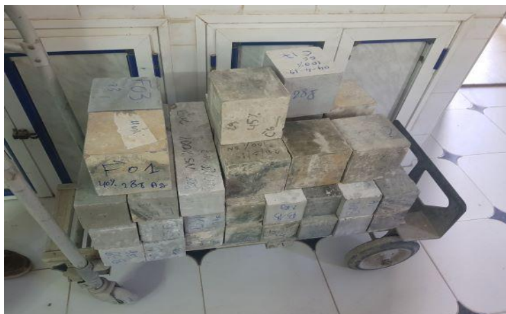
Figure 04: Sampling of Concrete Test Specimens.
