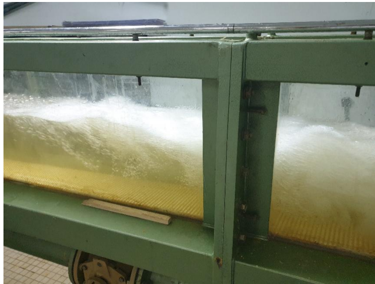
Photograph. 3. Hydraulic jump moving through a rough-bottomed canal.
