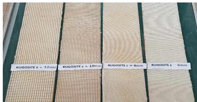
Photograph. 2. Different roughnesses tested.
