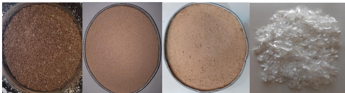
Oil Wells Sand (OWS) Dune Sand (DS) Alluvial Sand (AS) polypropylene Fibers
