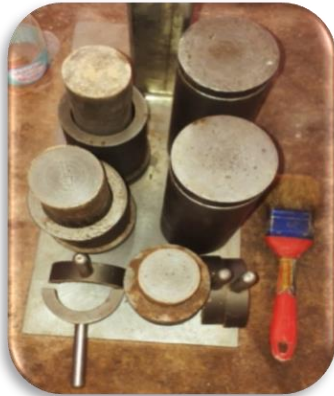
Figure.7 molds for making the specimens
