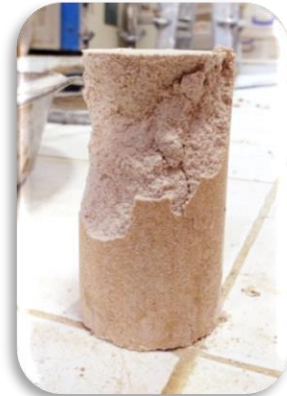
Figure.9 specimen after crushing
