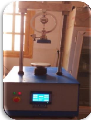
Figure.8 crushing hydraulic press used to measure the compressive strength of the specimens.
