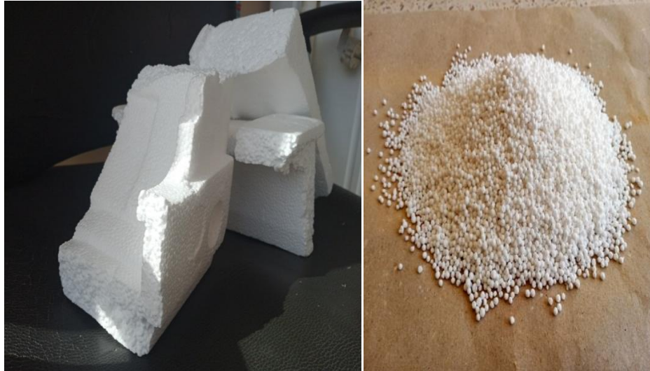
Fig.8. Polystyrene waste and polystyrene granules
