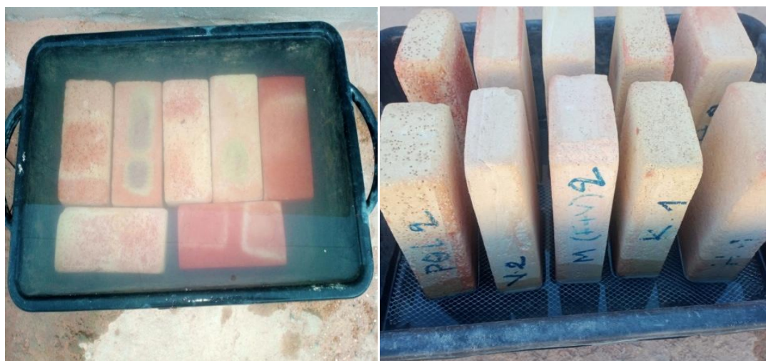
Fig.12. Total and capillary water absorption test
