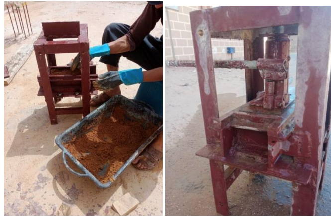
Fig.9. Pressure device used to perform samples.
