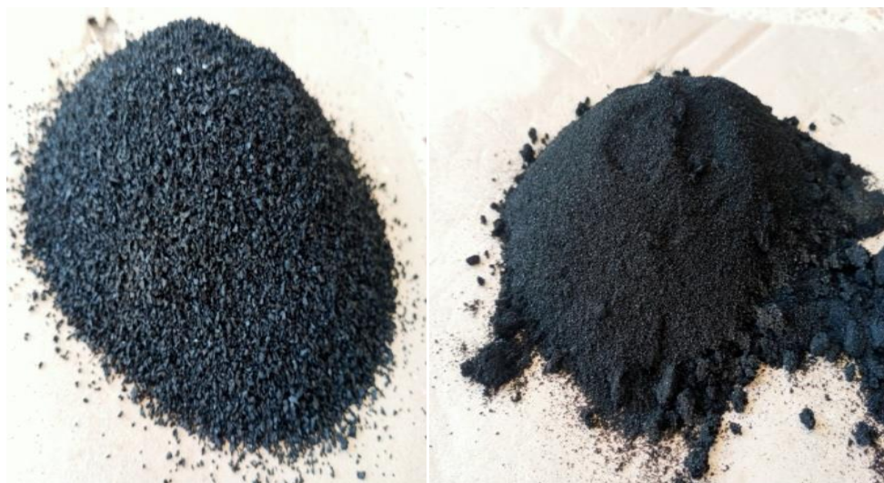
Fig.4. Synthetic rubber granules and powder
