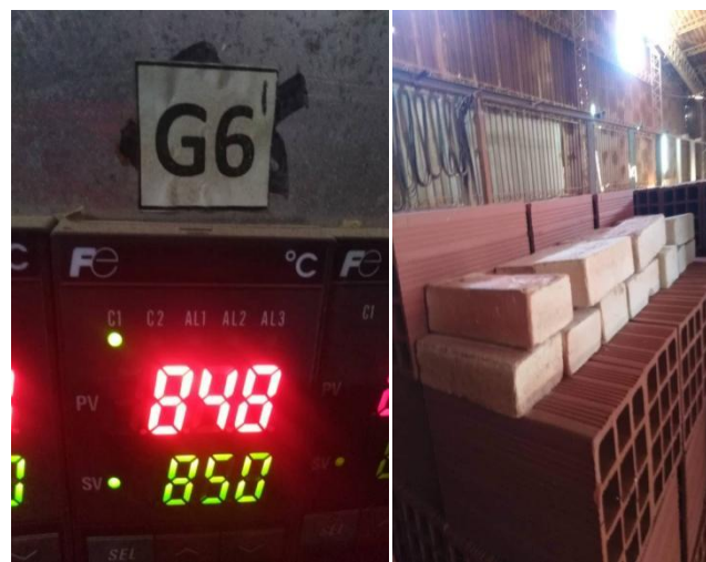
Fig.10. Burning samples in a tunnel furnace
