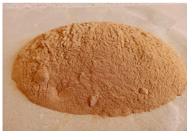
Fig.1. Clay powder used making samples
