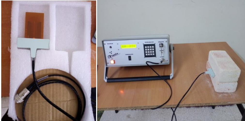
Fig.11. The CT meter and its probe
