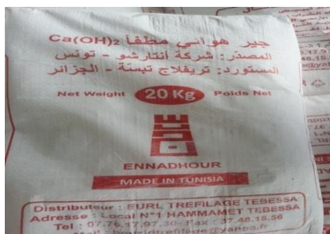
Fig.3. Used slaked lime to making samples
