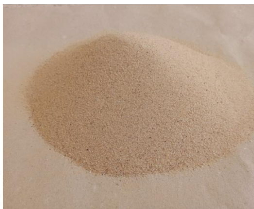
Fig.2. Used dune sand to making samples
