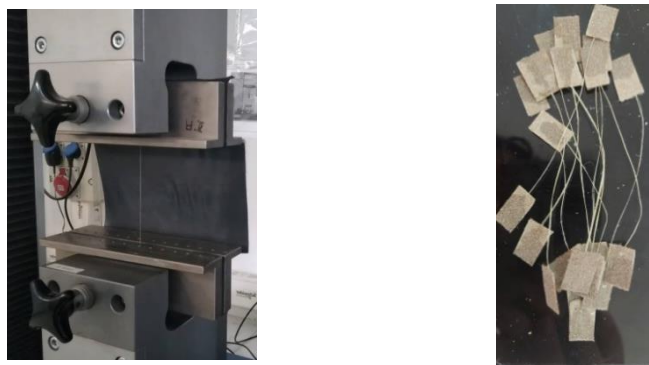
Picture 03: Date palm Spadix stem samples fibers mounted on a strip of paper for tensile testing
