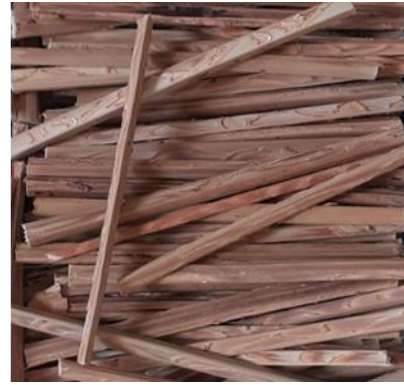
Figure 3: Multilayered date palm rachis(MDPR)
