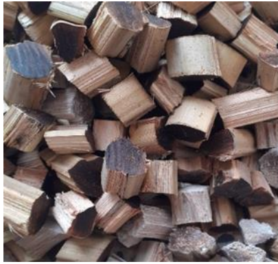
Figure 2: Granulated date palm rachis(GDPR)
