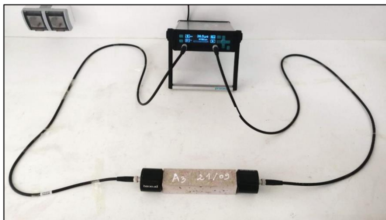
Figure 4. Ultrasonic Impulse Velocity Test.
