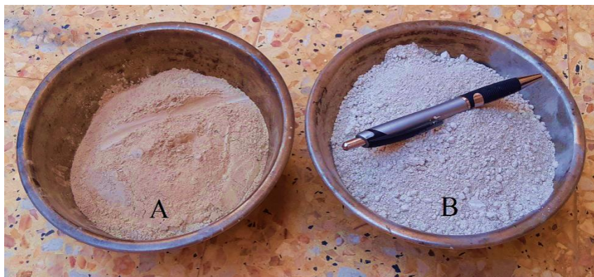
Figure 2: Filler used in study; A: limestone filler, B: rushed dune sand.
