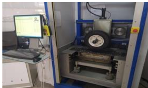
Figure 7. Photo of the wheel track test and wheel track test apparatus.
