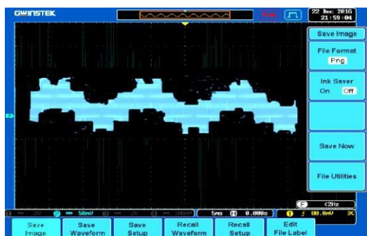
Fig. 24a – Inverter output voltageof PID methods .
