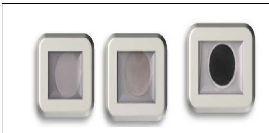
Figure6. Examples of filters taken for PCDD / F analysis
