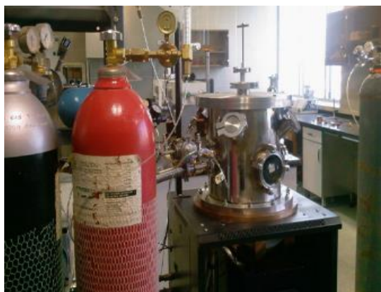
Fig. 2 Iranian Sun plasma focus device
