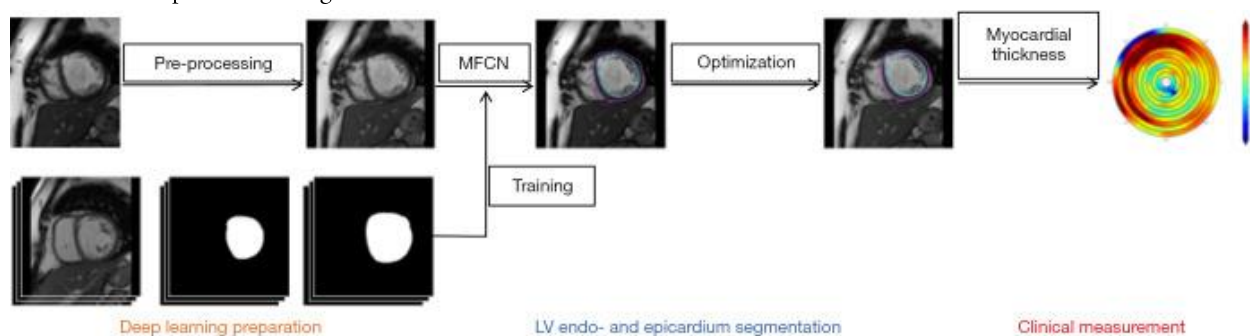
Figure 2: Schematic illustration representing the modified UNET technique for segmenting the left ventricle's epicardial and endocardial outlines.
