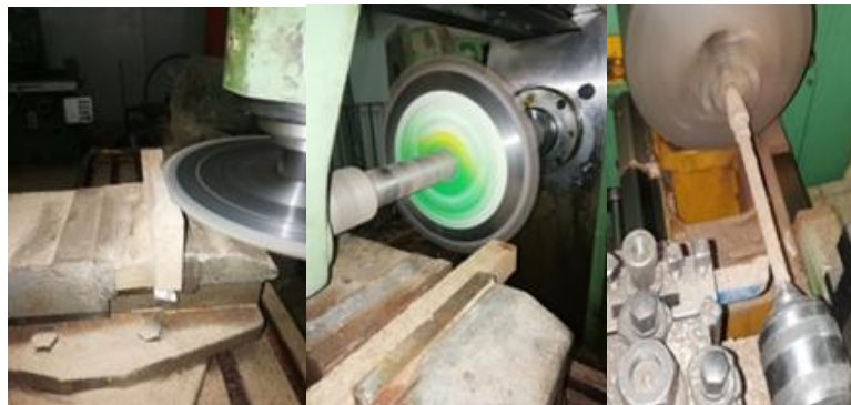
Figure 4. Cutting the Test specimen (a) traction, (b) compression, (c) fatigue
