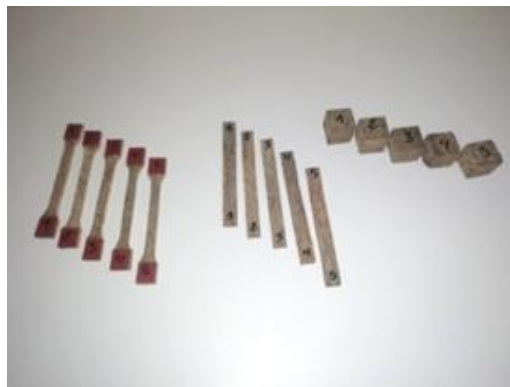
Figure 5. Test peciment for bending, traction, compression and fatigue.
