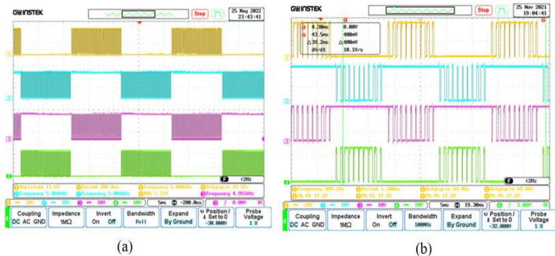
Figure IV 15: Unipolar PWM control signals: (a) for 5 kHz, (b) for 2.5 kHz.
