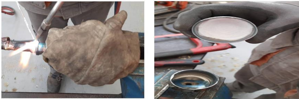
Fig.20.Photo of filter drier, (A) the correct welding method, (B) the inner part of the filter drier after welding
