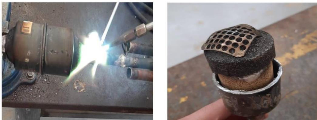
Fig.20.Photo of filter drier, (A) the correct welding method, (B) the inner part of the filter drier after welding
