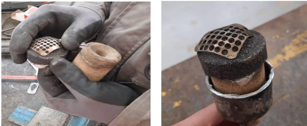
Fig.19. Photo of a damaged internal section of the filter drier
