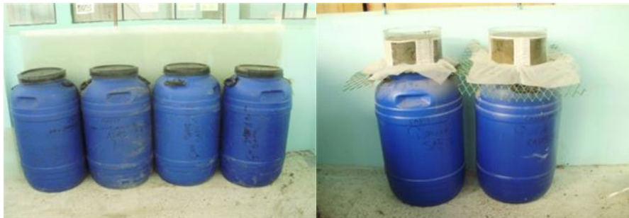
Photo 1 Natural air drying of sediment from Casablanca and Safi quays
