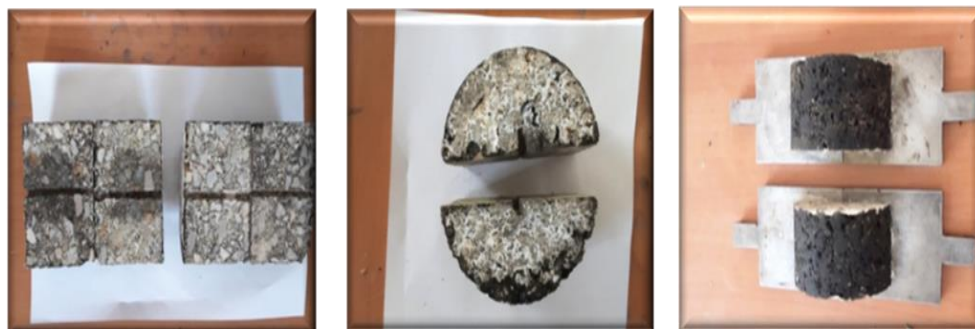
Cutting and gluing samples onto plates
