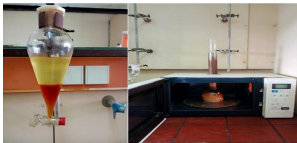
Fig.2. Experimental set-up of microwaves irradiation in domestic modified microwave for production of biodiesel
