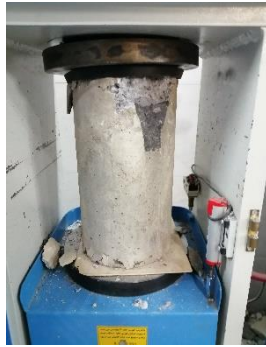
Figure 12. Rapture in repair concrete
