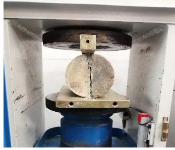
Figure 7. Rupture mode of repaired concrete specimen in an indirect tensile test
