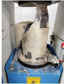
Figure 12. Rapture in the contact surface
