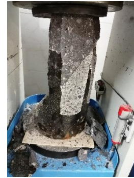
Figure 11. Rapture in old concrete
